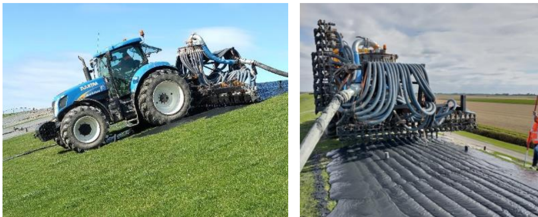
Figure 8 the usage of the manure injector to cover the dike
