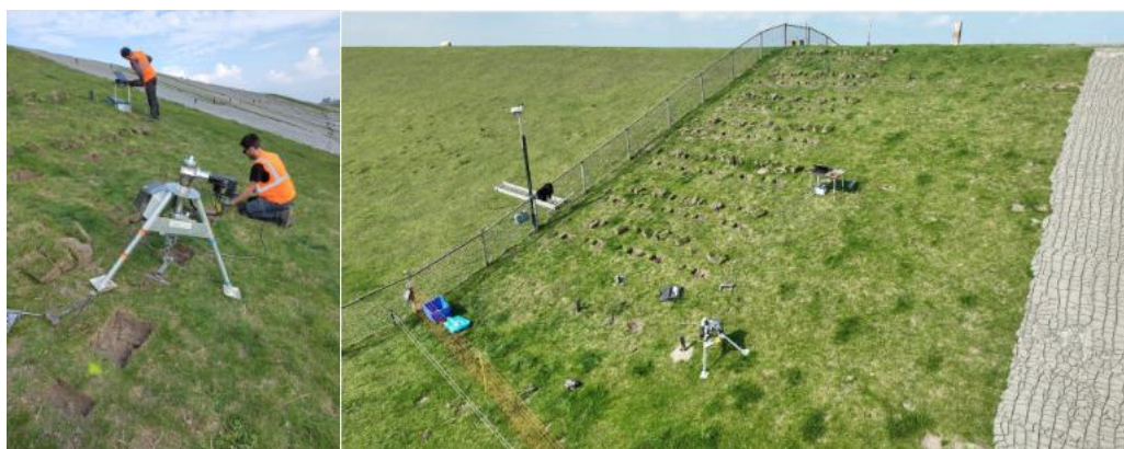
Figure 10 turf puller and 'results' of the test in the reference plot
