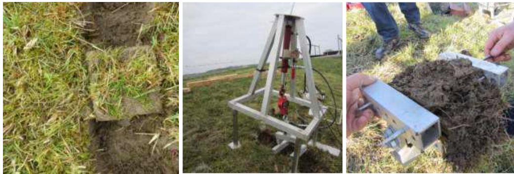
Figure 15 Different stages during the sod pulling tests: Top view condition 4 (left); Test set-up (middle); Pulled out sod (right)
