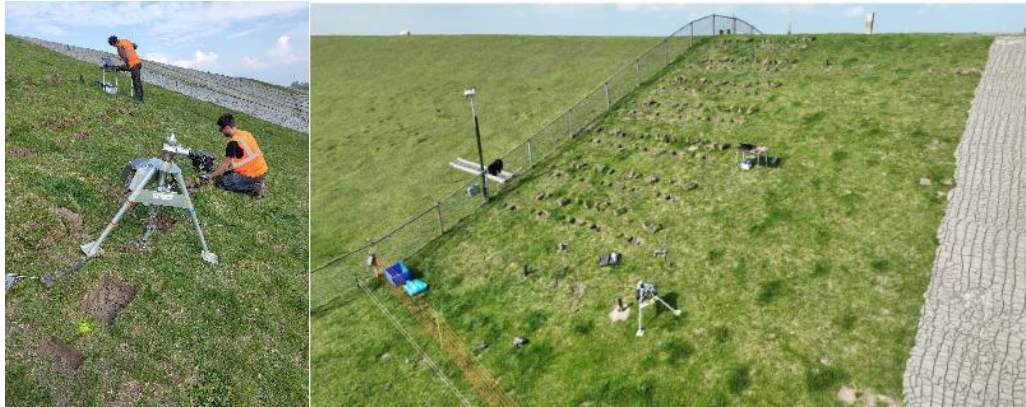
Figure 13 turf puller and 'results' of the test in the reference plot
