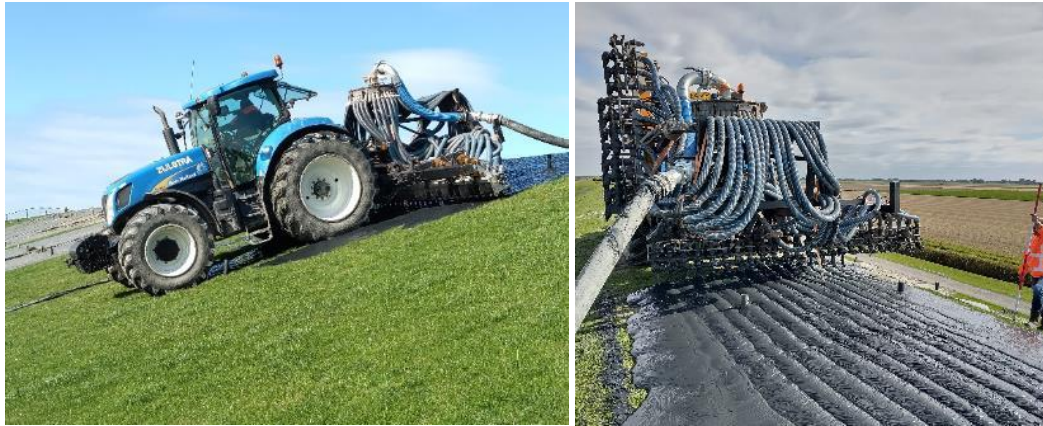
Figure 9 the usage of the manure injector to oversurface the dike
